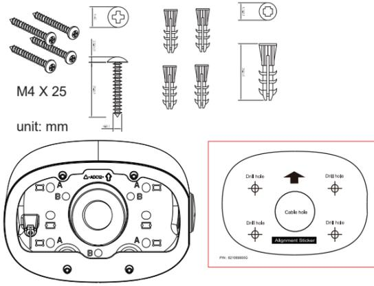
**A-2** Attach the included alignment sticker to a preferred position. Drill holes on the wall and install the tilt bracket. If the space behind the wall allows, you may also pass cables through the wall.
