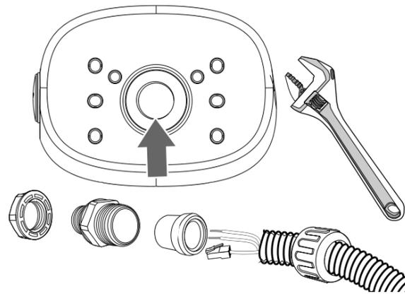
**B-3** Install the tilt bracket to AM-312 using the included M4 screws, washers and hex nuts. Pass the conduit through the center hole of the AM-312.
