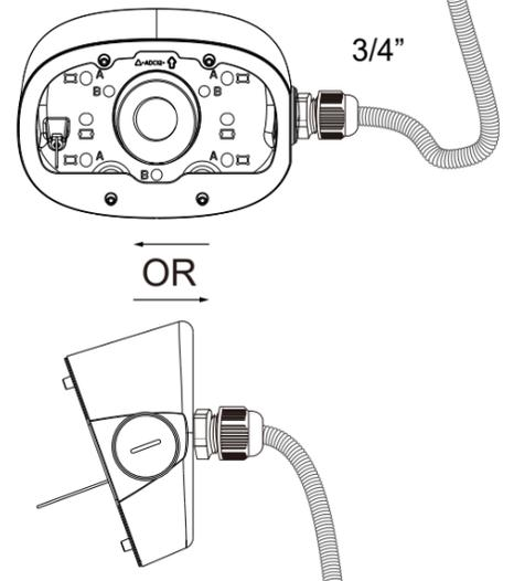
**A-6** Attach the waterproof cable gland to the retention clips at the back of the camera. Connect a grounding wire to the ground screw of the camera.
