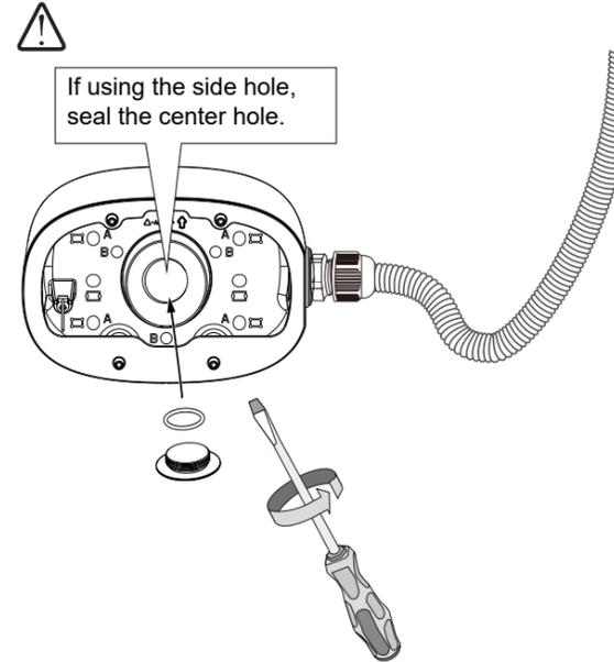
**A** Remove the plastic plug on the conduit hole. A 3/4" conduit is required for routing the cables with waterproof connection.
