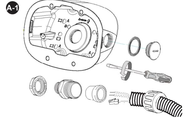
Install the cable gland and pass cables through it. The conduit is user-supplied.
